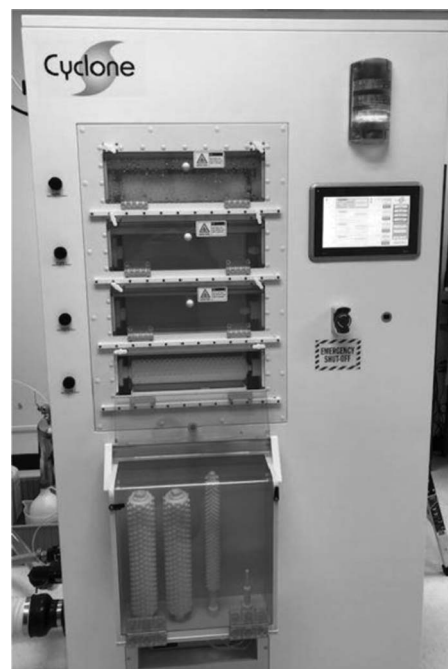
Figure 2. Cyclone brush processing system.
